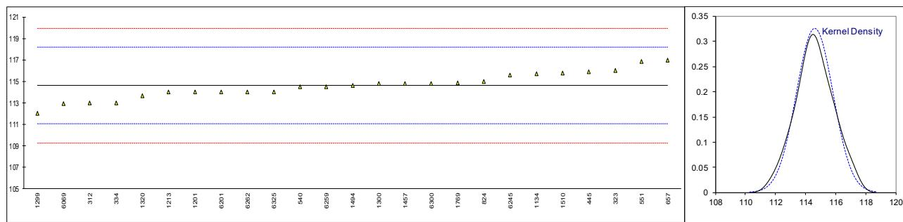
Determination of Kinematic Viscosity at 40°C on sample #20050; results in mm<sup>2</sup>/s
